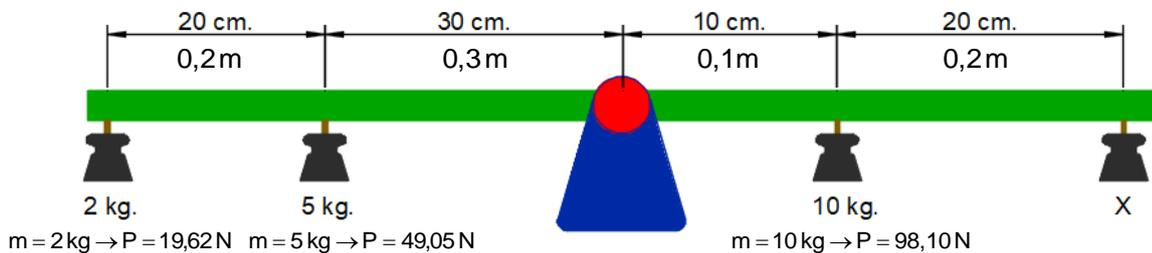
$$m = 2 \text{ kg} \rightarrow P = 19,62 \text{ N} \quad m = 5 \text{ kg} \rightarrow P = 49,05 \text{ N}$$
